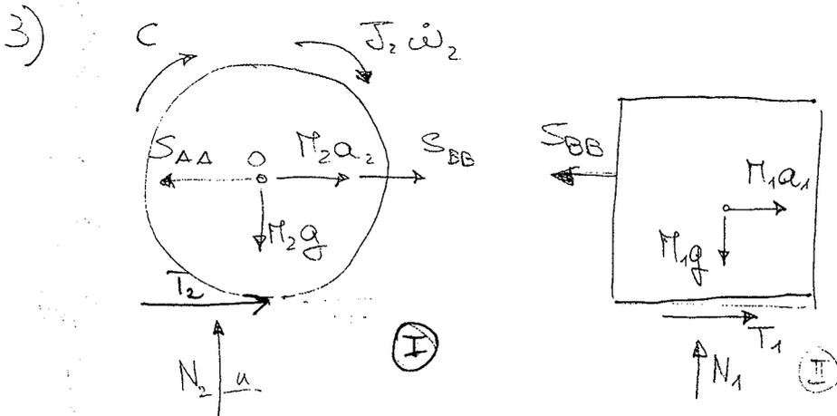
$$S_{BB} = M_1 a_1 + T_1 = M_1 R T_1 \dot{\omega}_m + f_d M_1 g$$
