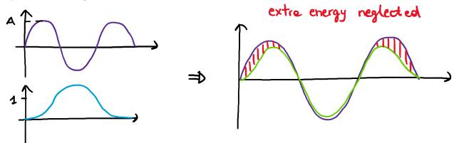
The function that I've chosen, and I have multiplied is called window. So, we can also define the window as a function that is able to removes the extra cycle in an original signal that is the main responsible for
