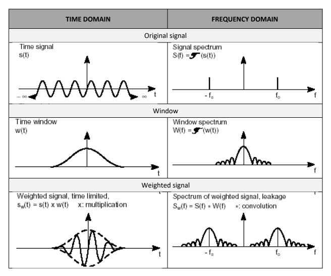
So, the shape of a window's spectrum is made of a lot of lobes. There is a main lobe which aim is to increase the effect of the interested frequency and then there are a lot of side lobes which main effect is to decrease the effect of the unexpected frequency.
