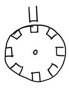
passing from a time domain acquisition to an angular space domain acquisition. We don't acquire anymore according to the time, but we are acquiring according to the angular position of the trigger. So, we must change the axial dimension of the acquisition from the time t, to the angles  $\alpha$ . The acquisition time will be swapped from T to bigger  $\alpha$  which is written as A. Of course, also the frequency resolution will change, as the following plots state:
