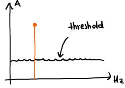
Until now we have done something which is not precise and coherent: we have talked about the average only in term of amplitude where we know that the output of the FFT is a complex number. So, until now we have completely neglected the complex part. Actually, in order to reduce the noise, is extremely useful to consider the all complex number which represent a vector.
