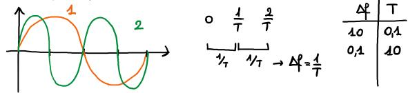
If I need a better frequency resolution  $\Delta f$ , I need to increase not the sampling frequency but the time acquisition. The frequency of sampling  $f_s$  is equal to the number of sampling  $n_s$  divided per the period T and so the link between these two quantities is:
